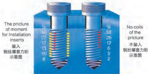
The diagram of moment of force 力矩示意图
