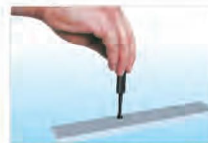
Take out the insert 取出钢丝螺套
